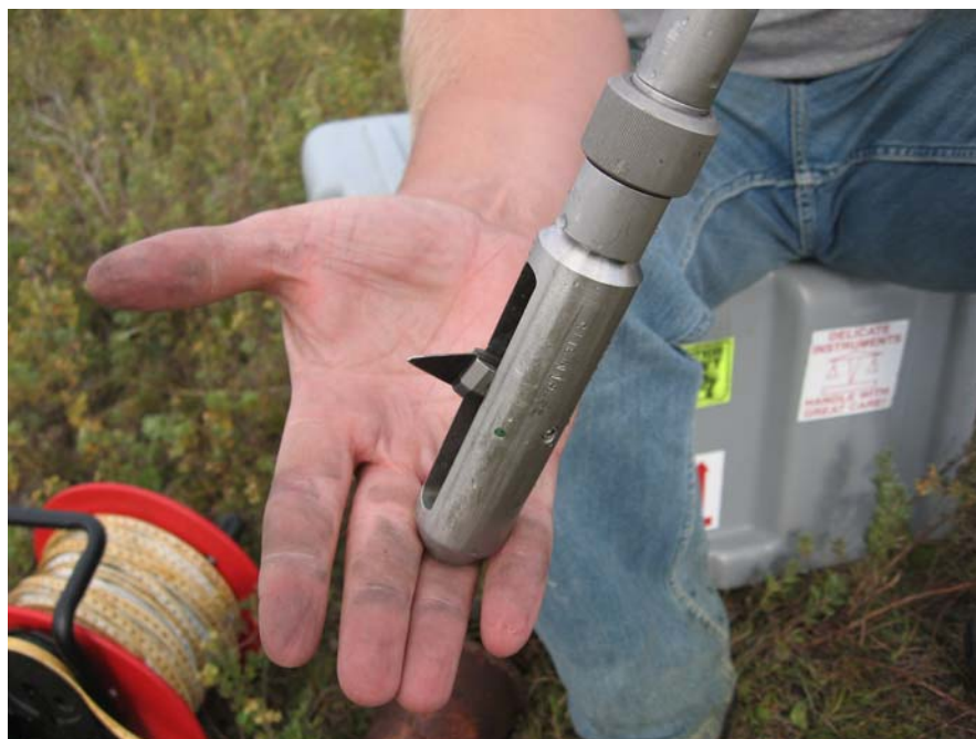
Figure 2 Packer Puncturing Tool Used to Deflate Packers in US-7
